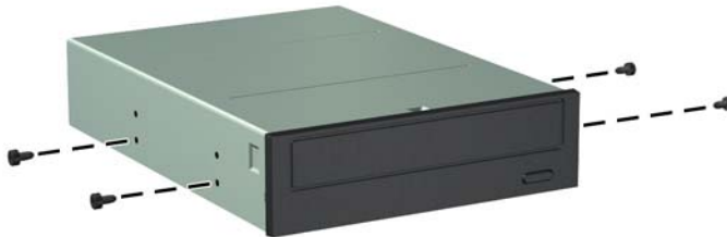
Figure 3-21 Installing Guide Screws (Optical Drive Shown)
